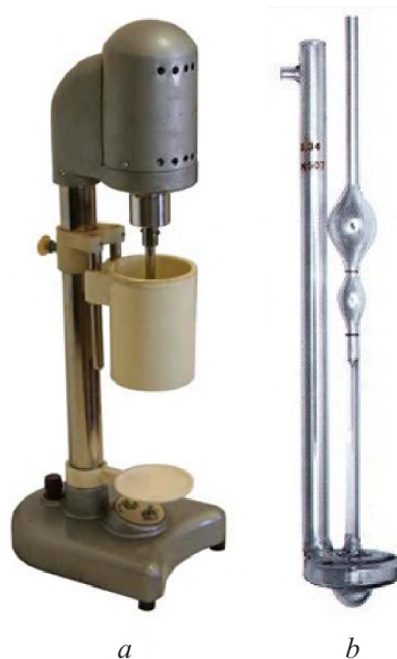
Fig. 1. The types of equipment, used during the study: a – micro-shredder of tissues RT-1; b – viscosimeter VTL-2 with capillary diameter 0,56 in water thermostat
