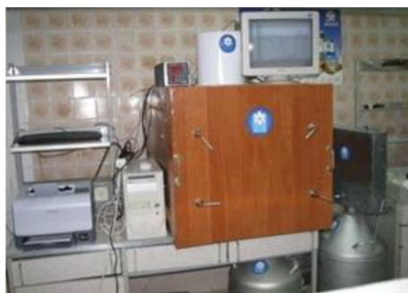
Fig. 1. Cryogenic program freezer with computer support
