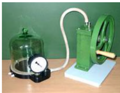
Fig. 14. Kamovsky electrovacuum pump with dilution 13 Pa
