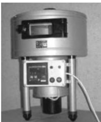
Fig. 5. Electric drying cabinet (EDC-3M (PE SumyCDDandA, Sumy, Ukraine)
