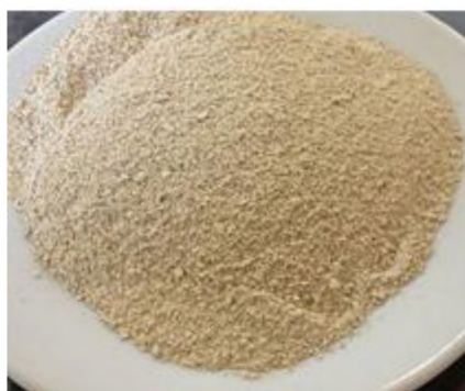
Fig. 4. Nanopowder of topinambour sublimation drying
