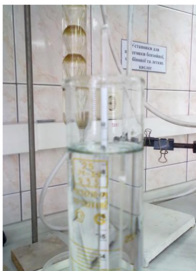
Fig. 1. Determination of strength of vodka of TM “Pervak” with help of glass alcoholmeter
