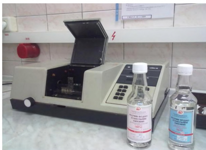
Fig. 3. Determination of mass concentration of aldehydes in special vodka of TM “Pervak”
