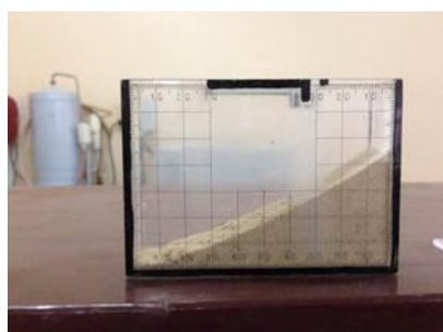
Fig. 10. Device for determination of natural slope angle
