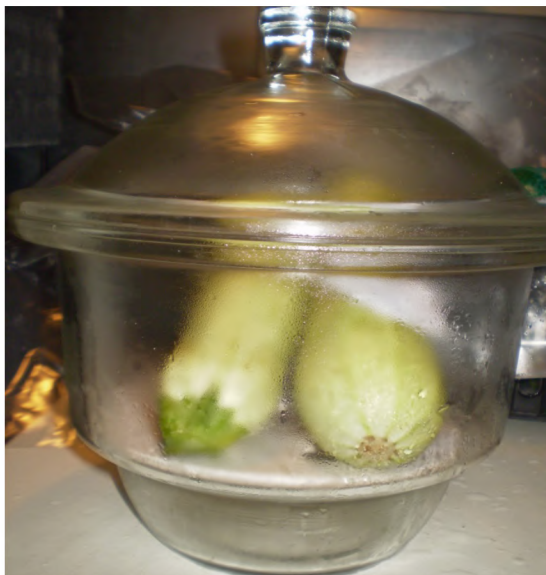
Fig. 3. Determination of vegetables respiratory rate by Tolmachev's method
