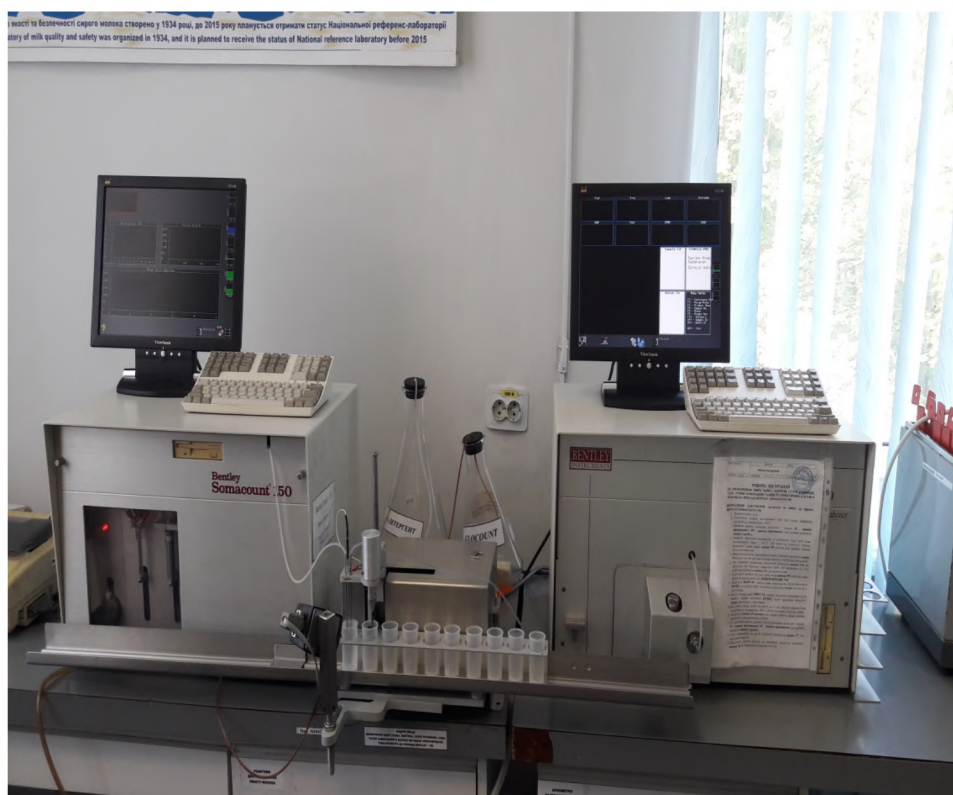
Fig. 1. device for determination of somatic cells «Bentley Somacount 150» (on the left) and for determination of physical-chemical composition of goat milk «Bentley Instrumenis» (on the right) (USA)
