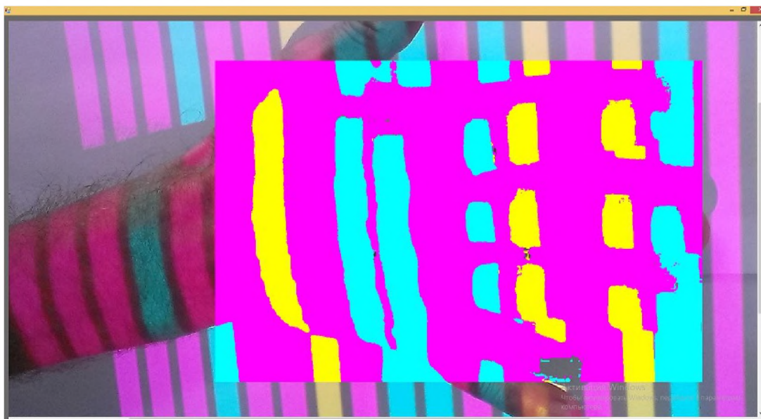
Fig. 9. Determination of the dominant color of the CMY illumination
