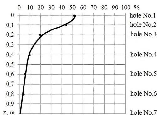
Fig. 9. Mass distribution of contaminants at the filter height after 20 hours of its operation
