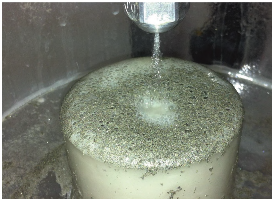
Fig. 8. The bubble-particle aggregates formed by in UP at CF tests (modified from [2])
