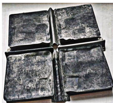
Fig. 2. Residual thermal deformations of workpieces
